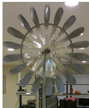
Figure 1. The first version of the windmill turbine with blades made of thin flexible steel sheet.
